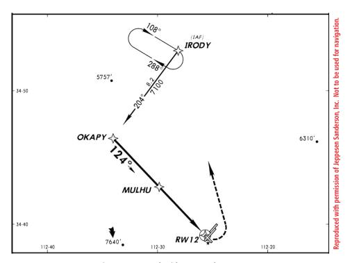
Figure 1 Approach with No Procedure Turn
