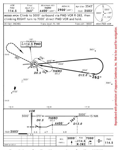
Figure 5 Course from Fix to Distance or Course from Fix to DME Distance
