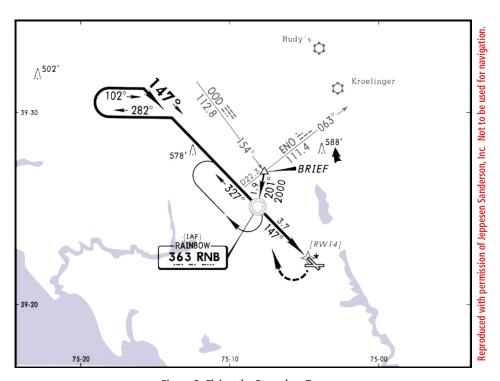
Figure 2 Flying the Procedure Turn
