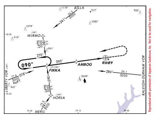
Figure 4 Flying an Approach with a Hold
